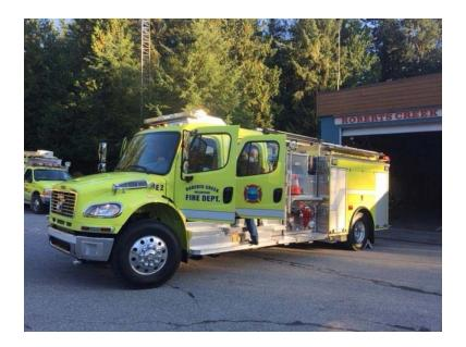
Engine 2: This apparatus is a full Class "A" Type I pumper with a 1000 gallon tank supplying a 1050IGPM pump. It serves as the frontline pumper carrying up to 5 firefighters to the incident scene. E2 is built on a Freightliner chassis with a Crew Cab as open rear seating is no longer permitted in new construction. Increased scene lighting increases the safety of evening responses. Other Firefighter safety features have been added to comply with current NFPA standards.
