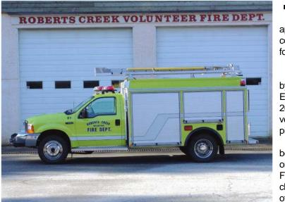
Engine 1: This apparatus is a compressed air foam system (CAFS) manufactured by Hub Fire Engines in 2000. It is a very versatile piece of apparatus being built on a one ton Ford F550 4x4 chassis. This offers a great
