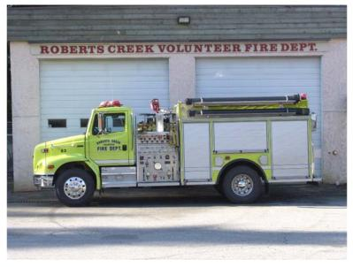
Engine 3: This apparatus is a full Class "A" Type II Pumper and fills our for need а tanker as it carries almost 1300 gallons of water. It also has a foam injection system and carries 30 gallons of foam concentrate. Engine 3 is built
